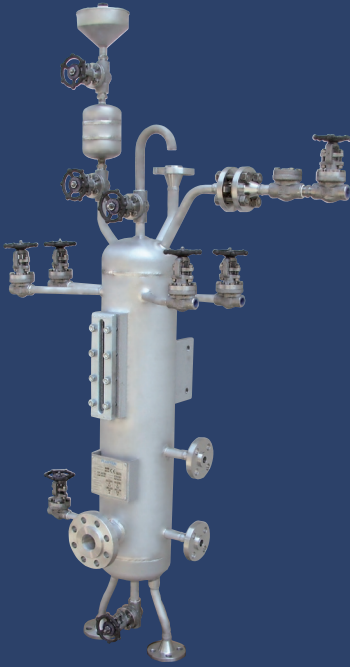
Barrier tank for Plan 53A with flanged connections, refilling device and temperature gauge connection according standard API 682
