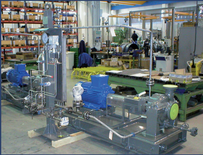
Double pressurized seal on API 610 heavy duty centrifugal pump with Plan 53B system
